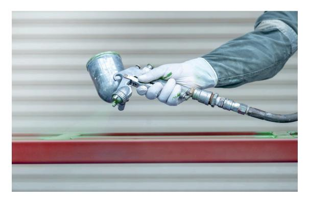
In addition to traditional painting methods, modern painters must master contemporary techniques like paint spraying. Paint spraying training courses teach the use of spray equipment, which is essential for large-scale projects and specific finishes. Paint sprayer training encompasses equipment maintenance, spray patterns, and safety protocols,
